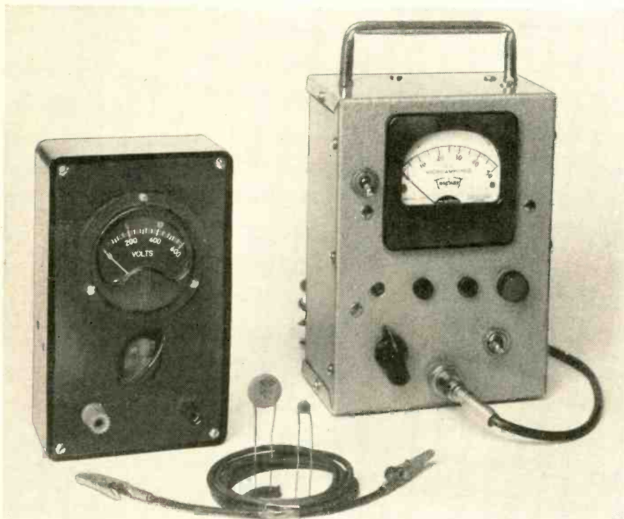
Bias box (left), dc vtm, clip leads and ceramic capacitors are all you need to tame the video if.
