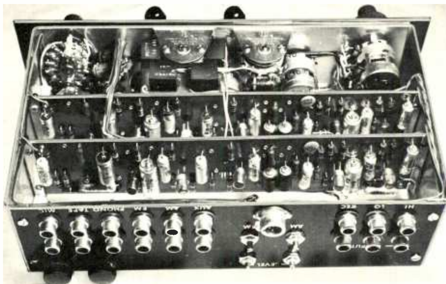
Underchassis view of preamp. Angle brackets fasten the circuit boards to ends of chassis frame.
