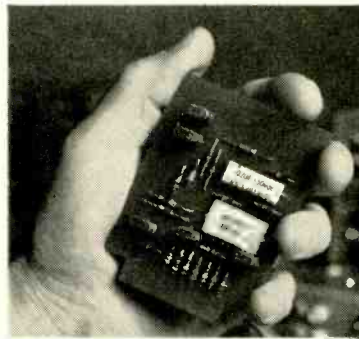
A single artificial neuron. It delivers electrical impulses when stimulated, like a living cell. Neurons are also being used for research into hearing.
