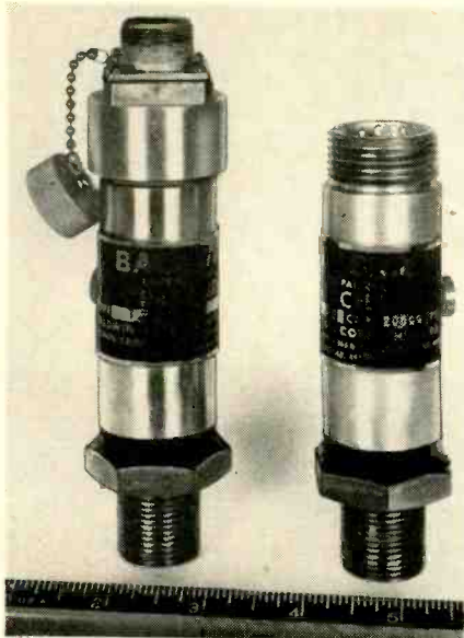
Fig. 6—The Baldwin SR-4 fluid pressure cell.
