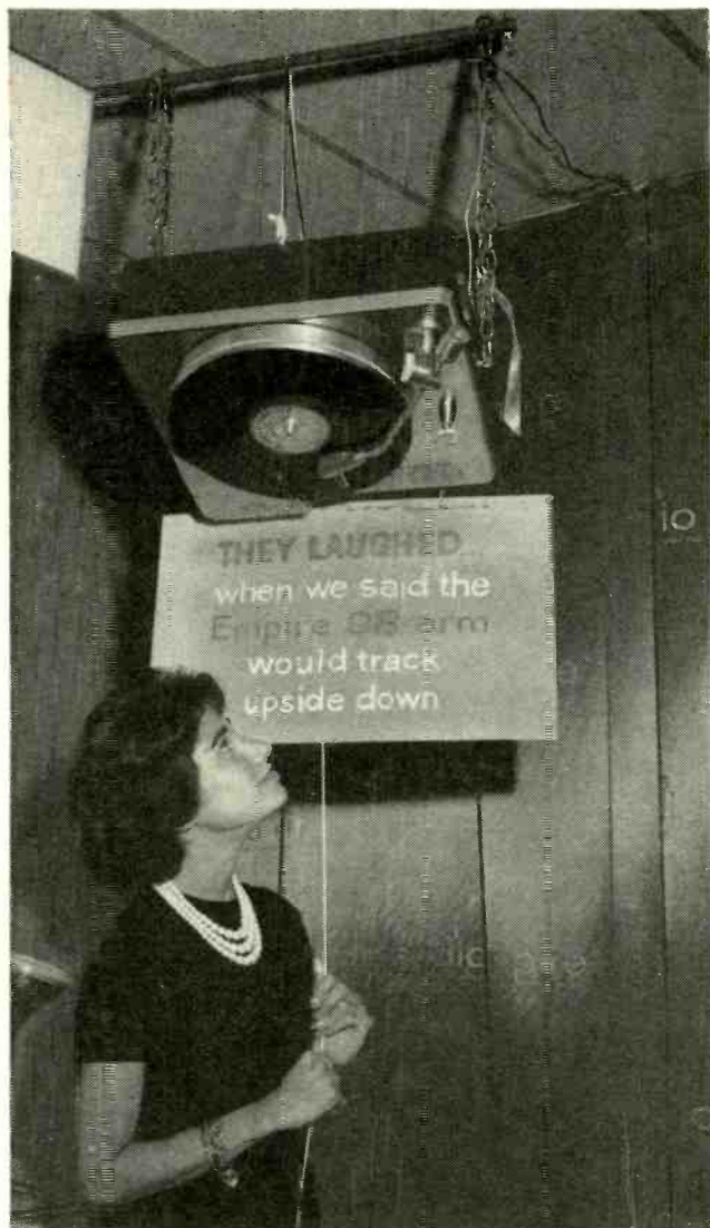
The upside-down record player operating. Empire's Gale Guterman is varying the stylus angle by a very simple means.
