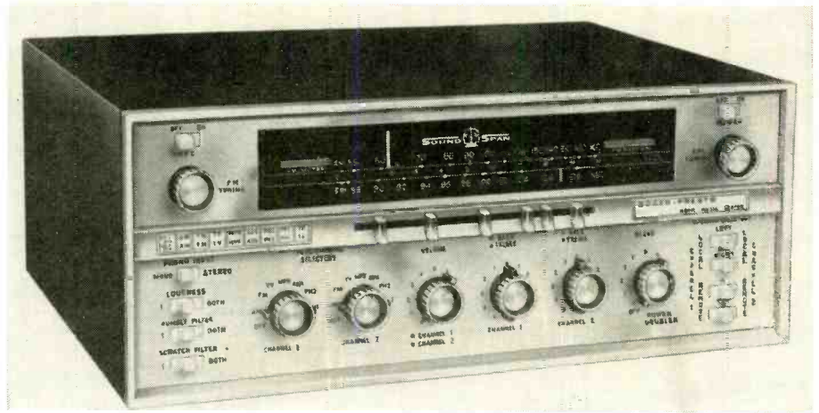
The Bogen RP-40. Unit consists of AM-FM stereo tuner, stereo preamp and dual power amplifiers. The amplifier system is also available without the tuner.
